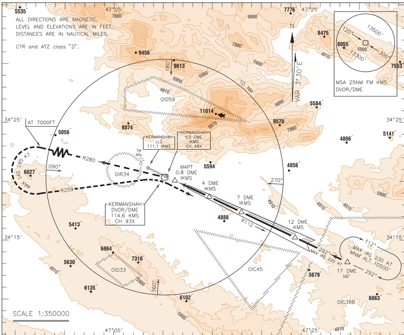
MISSED APPROACH: At 0.8 DME (IKMS) climb straight ahead to DVOR/DME, then climb on RDL 280 to 7000 FT, then turn left (MAX IAS 185 KT) climb on RDL 259 to DVOR/DME and continue climb on RDL 113 to rejoin HLDG at 10500 FT.
