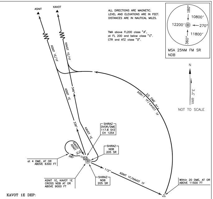
DEP RWY 29L/R - After take off turn left climb on BRG 290° to 6300 FT or above, then turn right (at 4 DME) to cross SR NDB at or above 9000 FT, then turn left to establish BRG 346° to KAVOT and climb to cleared level.
